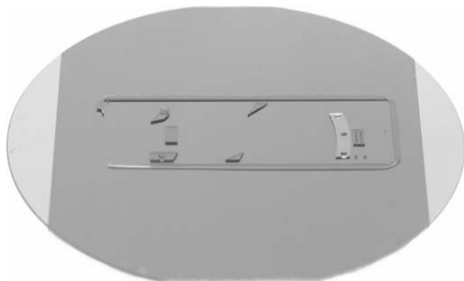
Fig. 4. SU-8 structures on 125\ \mu\text{m} Kapton ® release layer for later examinations with AFM
